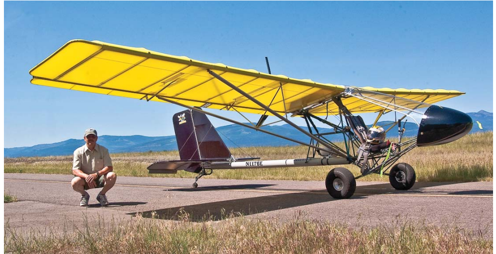
The Stinger Ultralight RANS S-7 kit. All parts fabricated. Some drilling and riveting. No welding, painting of fabric work required. Bob Greene coated the fabric with an ultraviolet protector.
